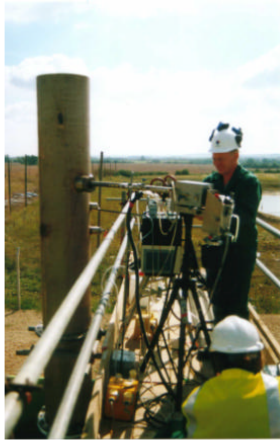
FIGURE 3. SAMPLING PLATFORM INSTALLED ACROSS A CONTAINERISED GENERATING SET, AND CLOSE-UP OF PARTICULATE SAMPLING EQUIPMENT INSTALLED ON SCAFFOLDING
