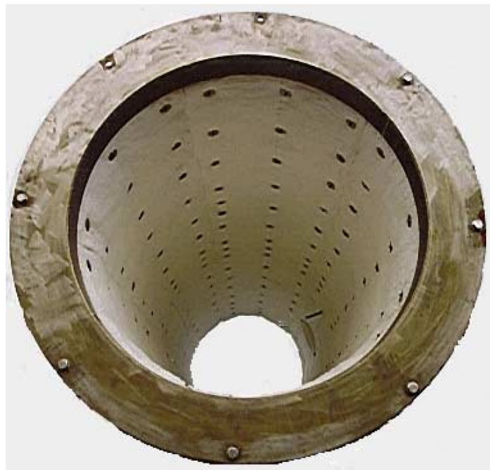
Internal view of a high temperature flarestack for landfill gas combustion.
